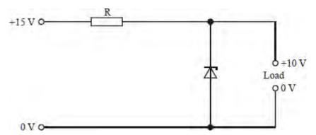
The maximum output current supplied to the load is 100 mA. The zener diode must have a minimum current of 10 mA passing through it to maintain its voltage.
