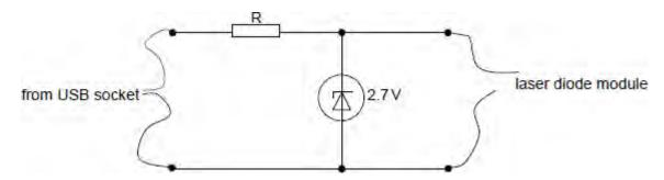
Specifications for the laser diode module and the USB output are:
